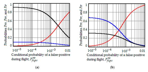
**Figure 6.** Dependences of the posterior probabilities of dismounting the LRU due to the in-flight false-positive (red curve), intermittent fault (black curve), and permanent failure (blue curve) on the conditional probability of in-flight false-positive when  $\lambda = 10^{-4} \text{ h}^{-1}$ ; (a)  $\theta = 1 \times 10^{-3} \text{ h}^{-1}$ ; (b)  $\theta = 1 \times 10^{-4} \text{ h}^{-1}$ .
