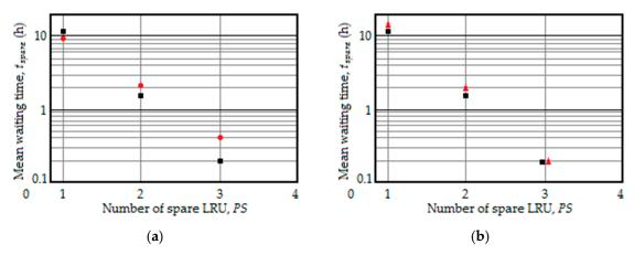
**Figure 9.** Dependences of the mean waiting time on the number of planned spare LRU (*PS*) for the second WM option; (a) , red circles:  $P_{flight}^{FP} = 1 \times 10^{-4}$ , black squares:  $P_{flight}^{FP} = 1 \times 10^{-3}$ ; (b)  $P_{flight}^{FP} = 1 \times 10^{-4}$ , black circles:  $\theta = 1 \times 10^{-4}$  h<sup>-1</sup>, red triangles:  $\theta = 1 \times 10^{-3}$  h<sup>-1</sup>.
