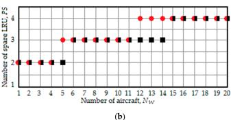
**Figure 10.** The dependency of the optimal quantity of spare LRU on the quantity of aircraft for the second WM option; (a) Red circles:  $P_{flight}^{FP} = 1 \times 10^{-4}$ , black squares:  $P_{flight}^{FP} = 1 \times 10^{-3}$ ; (b) Red circles:  $\theta = 1 \times 10^{-4}$  h<sup>-1</sup>, black squares:  $\theta = 1 \times 10^{-3}$  h<sup>-1</sup>.
