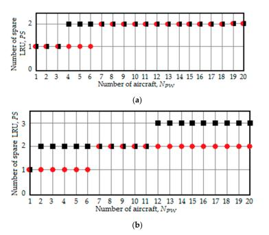
**Figure 14.** The dependency of the optimal number of spare LRU on the number of aircraft for the fourth and fifth PWM options; (a)  $\theta = 1 \times 10^{-4} \text{ h}^{-1}$ , red circles:  $P_{flight}^{FP} = 1 \times 10^{-4}$ , black squares:  $P_{flight}^{FP} = 1 \times 10^{-3}$ ; (b)  $P_{flight}^{FP} = 1 \times 10^{-4}$ , red circles:  $\theta = 1 \times 10^{-4} \text{ h}^{-1}$ , black squares:  $\theta = 1 \times 10^{-3} \text{ h}^{-1}$ .
