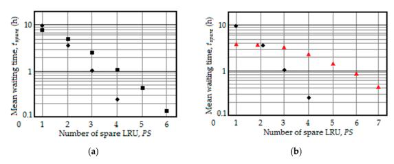
**Figure 3.** Dependences of the mean waiting time on the number of planned spare LRU (*PS*) for the first WM option; (**a**) circles:  $P_{flight}^{FP} = 1 \times 10^{-4}$ , squares:  $P_{flight}^{FP} = 1 \times 10^{-3}$ ; (**b**) black circles:  $\theta = 1 \times 10^{-4}$  h<sup>-1</sup>, red triangles:  $\theta = 1 \times 10^{-3}$  h<sup>-1</sup>.
