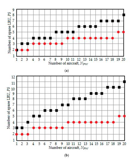
**Figure 11.** The dependency of the optimal quantity of spare LRU on the quantity of aircraft for the first PWM option; (**a**)  $\theta = 1 \times 10^{-4} \text{ h}^{-1}$ , red circles:  $P_{flight}^{FP} = 1 \times 10^{-4}$ , black squares:  $P_{flight}^{FP} = 1 \times 10^{-3}$ ; (**b**)  $P_{flight}^{FP} = 1 \times 10^{-4}$ , red circles:  $\theta = 1 \times 10^{-4} \text{ h}^{-1}$ , black squares:  $\theta = 1 \times 10^{-3} \text{ h}^{-1}$ .
