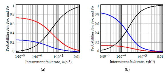
**Figure 7.** Dependences of the posterior probabilities of dismounting the LRU due to the in-flight false-positive (red curve), intermittent fault (black curve), and permanent failure (blue curve) on the intermittent fault rate when  $\lambda = 10^{-4} \, h^{-1}$ ; (a)  $P_{flight}^{FP} = 1 \times 10^{-3}$ ; (b)  $P_{flight}^{FP} = 1 \times 10^{-4}$ .
