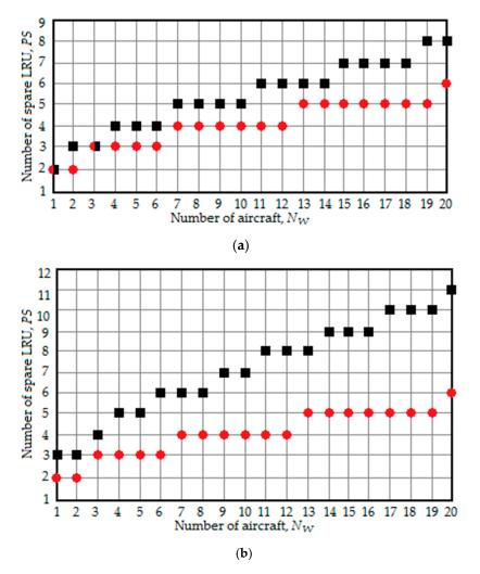
**Figure 4.** The dependency of the optimal quantity of spare LRU versus the quantity of aircraft for the first WM option; (a) Red circles:  $P_{flight}^{FP} = 1 \times 10^{-4}$ , black squares:  $P_{flight}^{FP} = 1 \times 10^{-3}$ ; (b) Red circles:  $\theta = 1 \times 10^{-4} \, \mathrm{h}^{-1}$ , black squares:  $\theta = 1 \times 10^{-3} \, \mathrm{h}^{-1}$ .
