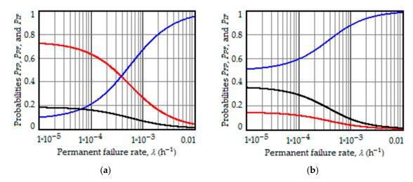
Figure 8. Dependences of the posterior probabilities of dismounting the LRU due to the in-flight false-positive (red curve), intermittent fault (black curve), and permanent failure (blue curve) on the permanent failure rate when  $\theta=10^{-4}~\mathrm{h^{-1}}$ ; (a)  $P_{flight}^{FP}=1\times10^{-3}$ ; (b)  $P_{flight}^{FP}=1\times10^{-4}$ .
