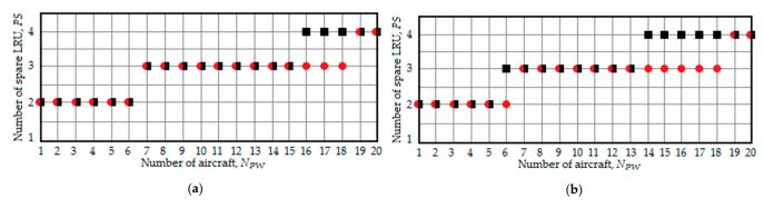
**Figure 12.** The dependency of the optimal quantity of spare LRU on the quantity of aircraft for the second PWM option; (a)  $\theta = 1 \times 10^{-4} \text{ h}^{-1}$ , red circles:  $P_{flight}^{FP} = 1 \times 10^{-4}$ , black squares:  $P_{flight}^{FP} = 1 \times 10^{-3}$ ; (b)  $P_{flight}^{FP} = 1 \times 10^{-4}$ , red circles:  $\theta = 1 \times 10^{-4} \text{ h}^{-1}$ , black squares:  $\theta = 1 \times 10^{-3} \text{ h}^{-1}$ .
