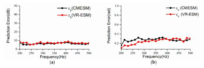
**Figure 17.** Prediction errors of sound pressure and phase at different frequencies ( $h_U = 0.2 \text{ m}$ ). (a)  $\varepsilon_p$  and (b)  $\varepsilon_{\Phi}$ .
