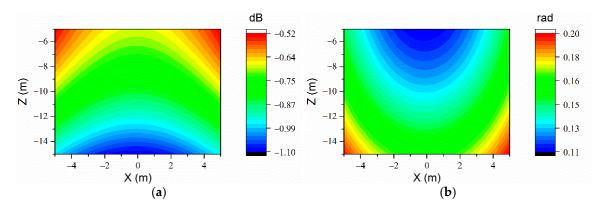
**Figure 5.** The sound prediction errors of ESM on the prediction plane in the free field at the frequency of 71 Hz (270uniform arranged measurement points determined by SVM). (a)  $p_E$  and (b)  $\varphi_E$ .
