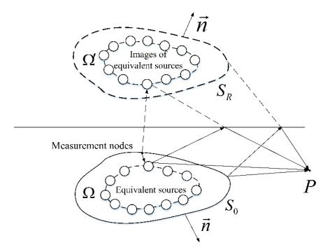
Figure 2. The schematic diagram of the equivalent source method in half-space.
