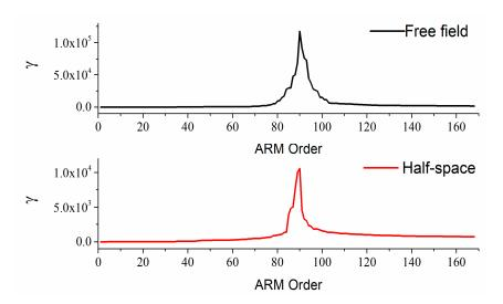
**Figure 8.** The variation of  $\gamma$  with the increase of ARM order when 90 uniform-arranged measurement points are used.
