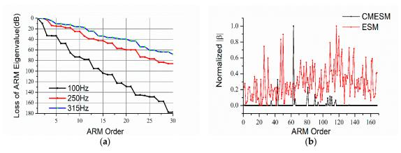
**Figure 7.** (a). Attenuation curves of ARM eigenvalues with the increase of the ARM order at different frequencies (unit: dB); (b) comparison of the normalized modal expansion coefficient sparsity between ESM and CMESM at the frequency of 100 Hz.
