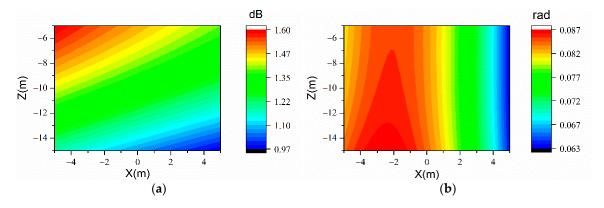
**Figure 6.** The sound prediction errors of ESM on the prediction plane when  $h_U = 0.2$  m at the frequency of 71 Hz (234 uniform arranged measurement points determined by SVM). (a)  $p_E$  and (b)  $\varphi_E$ .
