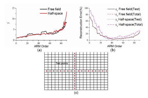
**Figure 12.** (a) The variation of  $\gamma'$  with the increase of ARM order, (b) the variation of reconstruction error versus the ARM order ( $f_0 = 71 \text{ Hz}$ ,  $h_U = 0.2 \text{ m}$ ), and (c) the arrangement of test points.
