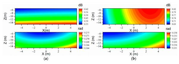
**Figure 11.** The sound prediction errors of CMESM on the prediction plane when 135 uniformly arranged measurement points are used at the frequency of 71 Hz. (a) Free field (L1 = 92, upper:  $p_E$ ; lower:  $\varphi_E$ ) and (b)  $h_U = 0.2$  m (L1 = 95, upper:  $p_E$ ; lower:  $\varphi_E$ ).
