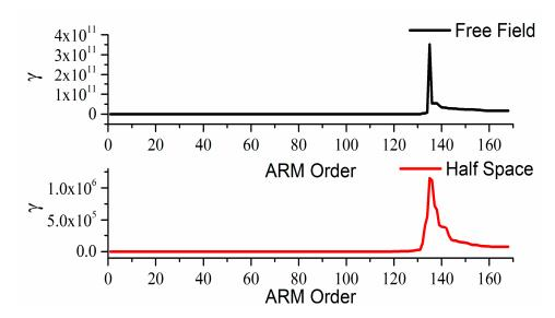
**Figure 10.** The variation of  $\gamma$  with the increase of ARM order when 135 uniformly arranged measurement points are used.
