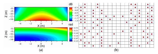
**Figure 14.** The sound prediction errors of VR-ESM on the prediction plane when  $h_U = 0.2$  m at the frequency of 71 Hz, L1 = 42. (a) Upper:  $p_E$ ; lower:  $\varphi_E$ . (b) The arrangement of measurement points (90 points optimized with EFI).
