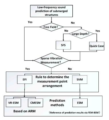
**Figure 1.** The flowchart illustrating the methodology of the paper. SFS, sound field separation; EFI, efficient independence; SVM, structural vibration mode; VR-ESM, vibration reconstruction equivalent source method; CMESM, compressed modal ESM; ARM, acoustic radiation mode; FEM, finite element method; BEM, boundary element method.
