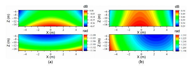
**Figure 9.** The sound prediction errors of CMESM on the prediction plane when 90 uniformly arranged measurement points are used at the frequency of 71 Hz. (a) Free field (L1 = 55, upper:  $p_E$ ; lower:  $\varphi_E$ ) and (b)  $h_U = 0.2$  m (L1 = 62, upper:  $p_E$ ; lower:  $\varphi_E$ ).
