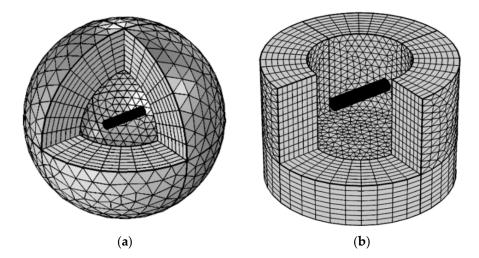
Figure 3. The sound radiation model for a structure: (a) free field and (b) half-space.
