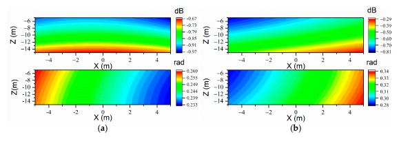
**Figure 16.** The sound prediction errors of CMESM on the prediction plane at the frequency of 71 Hz when 90 measurement points are used (optimized with EFI). (a) Free field (upper:  $p_E$ ; lower:  $\varphi_E$ , L1 = 66); (b)  $h_U = 0.2$  m (upper:  $p_E$ ; lower:  $\varphi_E$ , L1 = 75).
