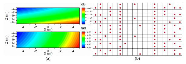
**Figure 13.** The sound prediction errors of VR-ESM on the prediction plane in the free field at the frequency of 71 Hz, L1 = 42. (a) Upper:  $p_E$ ; lower:  $\varphi_E$ . (b) The arrangement of measurement points (90 points optimized with EFI).
