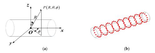
**Figure 4.** (a) The coordinate system for the structure; (b) the measurement points on the structural surface.
