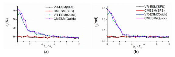
**Figure 19.** Prediction errors at different submerged depths in the SFS case and Quick case when 90 measurement points are used ( $h_U = 0.2 \text{ m}$ ,  $f_0 = 300 \text{ Hz}$ ). (a)  $\varepsilon_p$  and (b)  $\varepsilon_{\Phi}$ .
