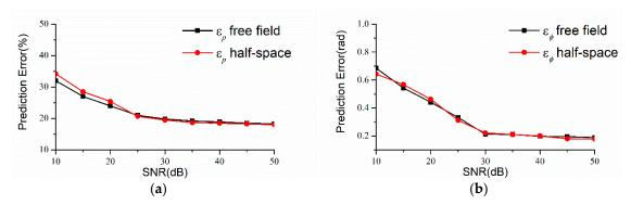
**Figure 18.** Prediction errors with the variation of the signal–noise ratio (SNR) ( $f_0 = 300$  Hz,  $h_U = 0.2$  m, 90 measurement points optimized with EFI). (a)  $\varepsilon_p$  and (b)  $\varepsilon_{\Phi}$ .
