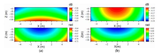
**Figure 15.** The sound prediction errors of VR-ESM on the prediction plane at the frequency of 71 Hz when 90 uniformly arranged measurement points are used. (a) Free field (upper:  $p_E$ ; lower:  $\varphi_E$ , L1 = 66); (b)  $h_U = 0.2$  m (upper:  $p_E$ ; lower:  $\varphi_E$ , L1 = 75).
